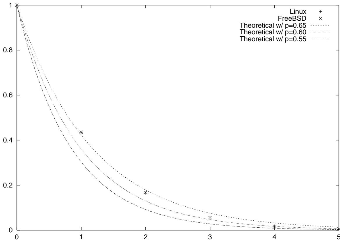
Figure 3: Strengthening with Randomized Nanosleeps. The theoretical curve has been refined from  $p^{2k+1}$  to  $p_0 p^{2k}$ , with  $p_0 = 1$ , because the attacker in these experiments can almost always win the first race.
