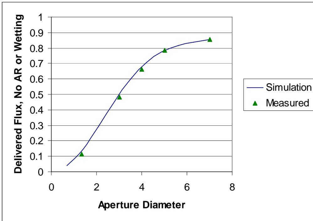
Figure 3: LightTools® Simulation versus Measured performance for the new coupler using a White LED
