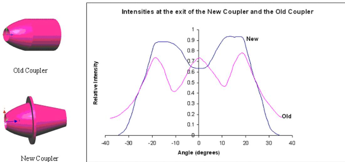
**Figure 4: Relative intensity distribution for Old and New couplers**
