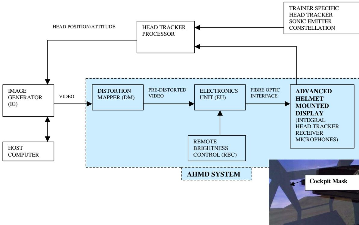
**Figure 2: System Block Diagram and Cockpit Mask**
