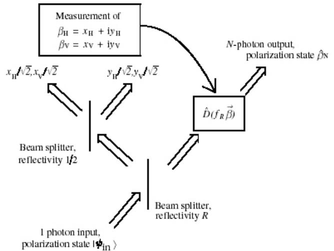
Figure 2: A Schematic of the optimal cloning set-up
