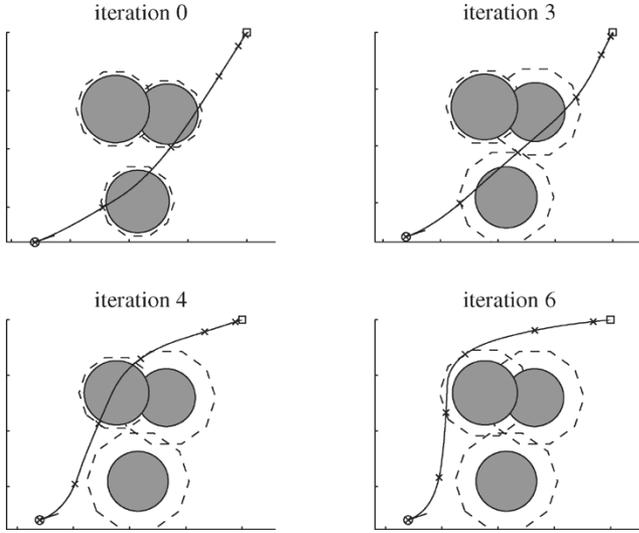
Fig. 5. Snapshots of the iterative MILP obstacle-growing algorithm. The circular regions denote obstacles, and the polygons denote the buffer regions used in the MILP formulation. Each cross denotes a time at which obstacle avoidance is enforced. For each iteration, there are five times at which obstacle avoidance is enforced ( $N_o = 5$ ).
