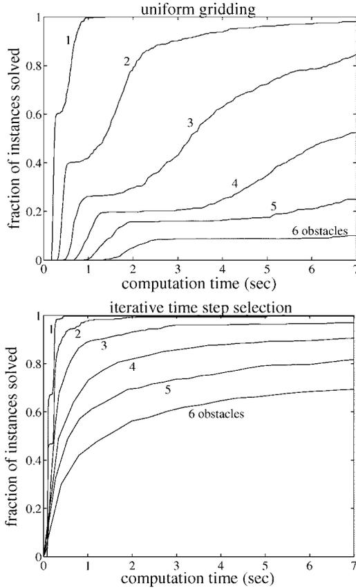
Fig. 7. Fraction of instances solved versus computation time for uniform gridding (top) and the iterative MILP time-step selection algorithm (bottom). We consider  $N_{\text{obst}} = 2, 3, 4, 5, 6$ . For each curve, 500 random instances were solved. The values of the parameters are  $N_u = 10$ ,  $M_u = 10$ , and  $M_o = 10$ .
