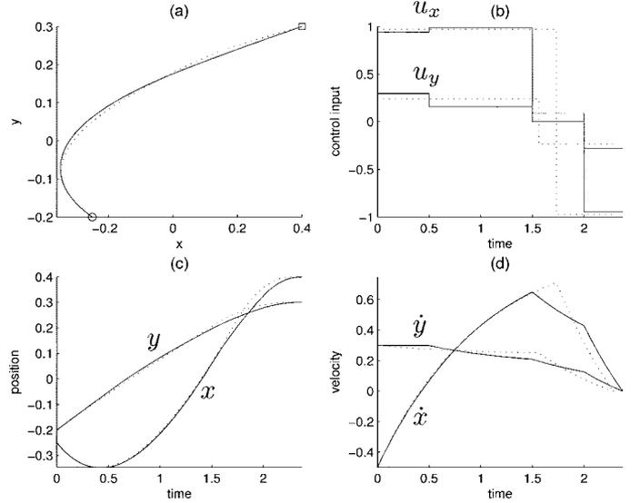
Fig. 9. Approximate time-optimal solution (solid lines) to an instance of the minimum-time vehicle-control problem of Section IV given by the iterative MILP algorithm. For comparison, we plot the near-optimal solution (dotted lines) for the continuous-time version of the problem obtained using techniques from [15]. The parameters are  $M_u = 20$ ,  $N_u = 10$ ,  $(x_s, y_s, \dot{x}_s, \dot{y}_s) = (-0.25, -0.2, -0.5, 0.3)$ ,  $(x_f, y_f, \dot{x}_f, \dot{y}_f) = (0.4, 0.3, 0, 0)$ .
