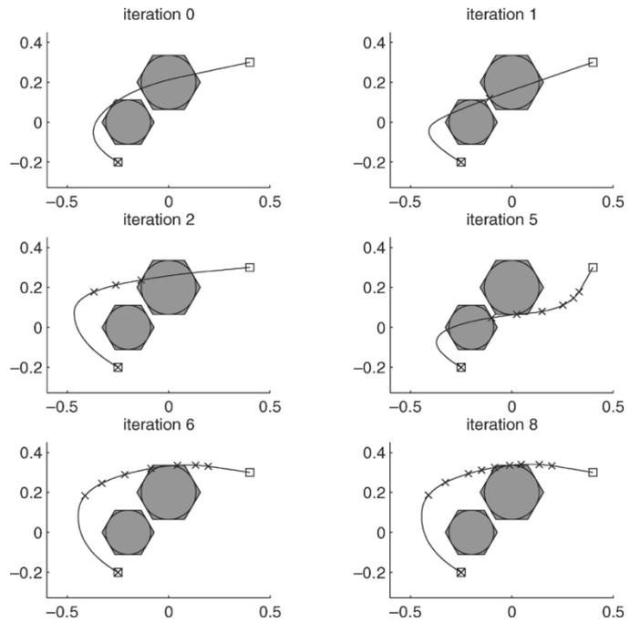
Fig. 2. Snapshots of the iterative MILP obstacle-avoidance algorithm. The circular regions denote the obstacles, and the polygons denote the buffer regions used in the MILP formulation. Each cross "x" denotes a time at which obstacle avoidance is enforced. The values of the parameters are  $M_o = 6$ ,  $M_u = 4$ ,  $N_u = 4$ ,  $(x_s, y_s, \dot{x}_s, \dot{y}_s) = (-0.25, -0.2, -0.5, 0.3)$ , and  $(x_f, y_f, \dot{x}_f, \dot{y}_f) = (0.4, 0.3, 0, 0)$ .
