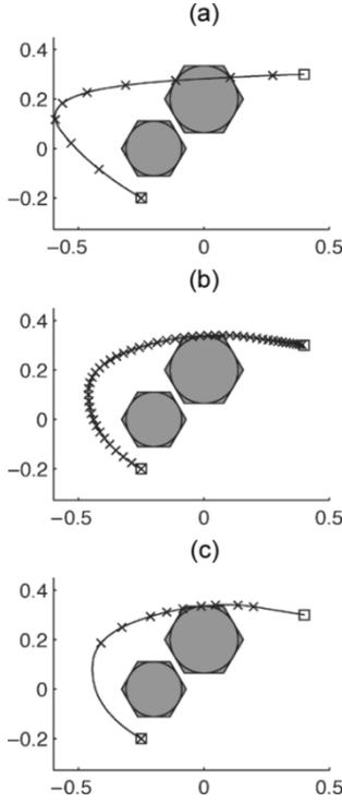
Fig. 1. (a) Resulting trajectory using uniform gridding ( $N_o = 10$ ). (b) Trajectory using a finer uniform gridding ( $N_o = 50$ ). (c) Trajectory using iterative MILP avoidance ( $N_o = 9$ ). The circles denote the obstacles, and the polygons denote the buffer regions used in the MILP formulation. The values of the parameters are  $M_o = 6$ ,  $M_u = 4$ ,  $N_u = 4$ ,  $(x_s, y_s, \dot{x}_s, \dot{y}_s) = (-0.25, -0.2, -0.5, 0.3)$ , and  $(x_f, y_f, \dot{x}_f, \dot{y}_f) = (0.4, 0.3, 0, 0)$ .
