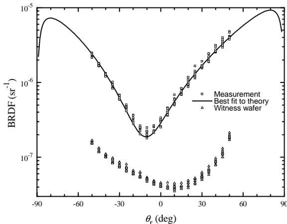
**Figure 3 Light scattering of p-polarized light by PSL spheres on a silicon substrate measured in the plane of incidence at five different locations (squares). The solid curve represents the best fit to the theory as described in the text.**
