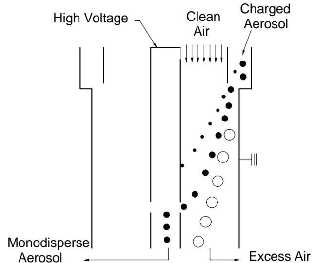
**Figure 2. A monodisperse aerosol is “selected” from a polydisperse aerosol based on the size dependence of the electrical mobility.**
