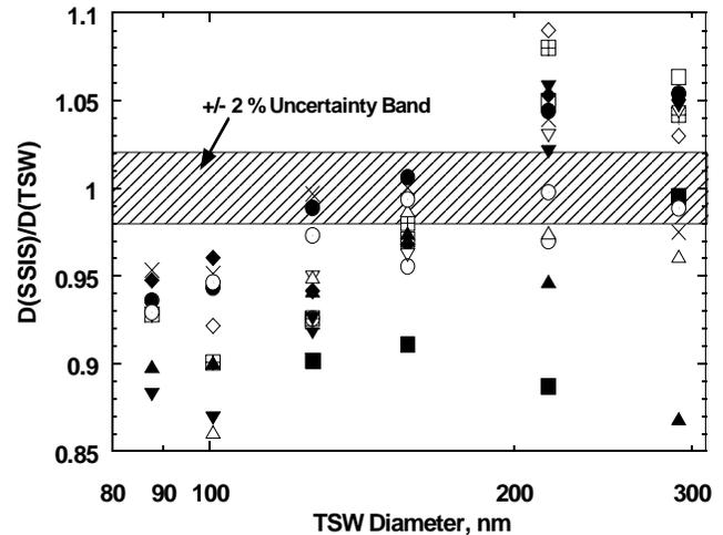
**Figure 1. The ratios of the SSIS diameters to those determined by TSW are plotted versus diameter for six calibration particles. Thirteen SSIS's were used at eight facilities for this study.**
