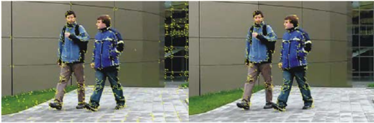
Fig. 1. Left – detected corners. Right – corners with detected motion
