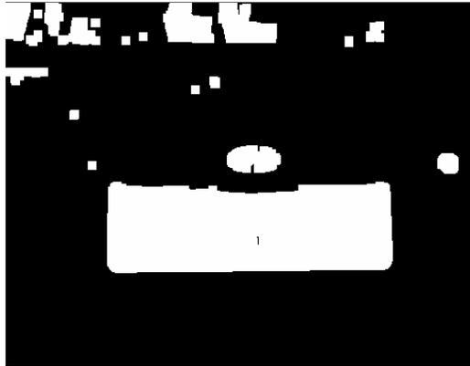
Fig. 4 Dilated image with a mask size of 9 by 9
