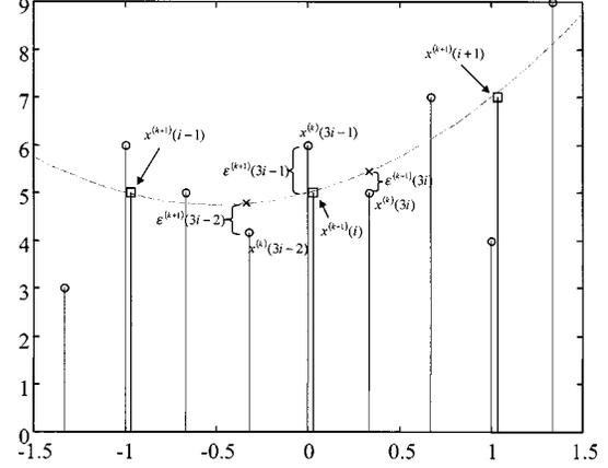
Fig. 2. Relationships between two consecutive shrunk signals. Shrunk signal values at scale  $k$  (circles); shrunk signal values at scale  $k+1$  (squares); prediction values from scale  $k+1$  to scale  $k$  (crosses); polynomial interpolation (dashed line).
