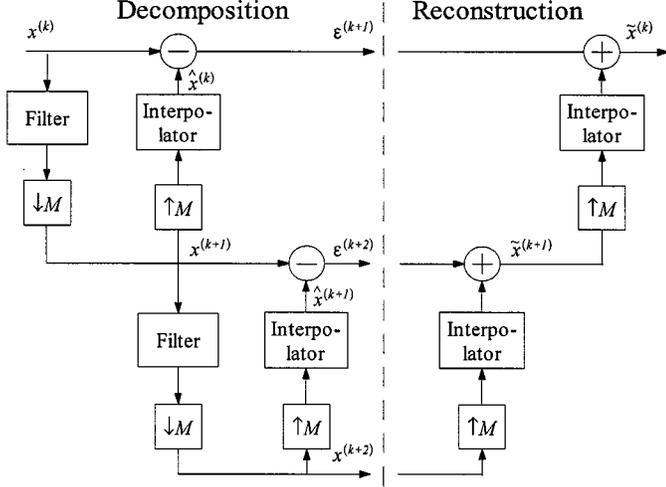
Fig. 1. General structure of a pyramid transform.
