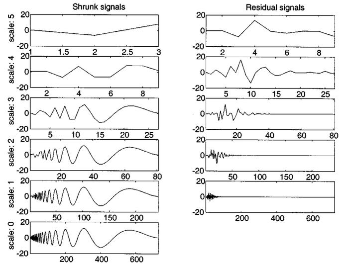
Fig. 3. ‘‘Doppler’’ signal decomposition using BMPT.
