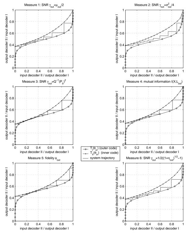
Fig. 2. Measures for tracing decoding convergence of serially concatenated codes (turbo decoding).
