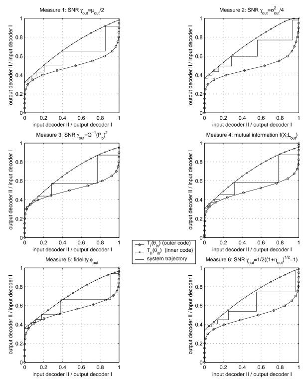
Fig. 4. Measures for tracing decoding convergence of iterative demapping and decoding (turbo BiCM).
