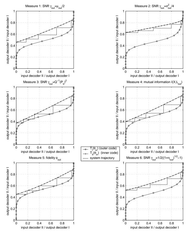
Fig. 3. Measures for tracing decoding convergence of iterative equalization and decoding (turbo equalization).
