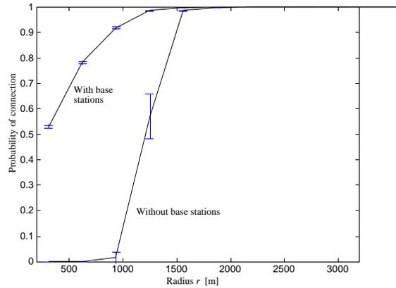
Fig. 11. Probability of connection in the region of Zurich without base stations and with base stations every 5km as a function of  $r$ .
