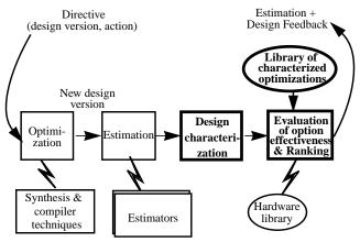
Fig. 2. Components of the design guidance system
