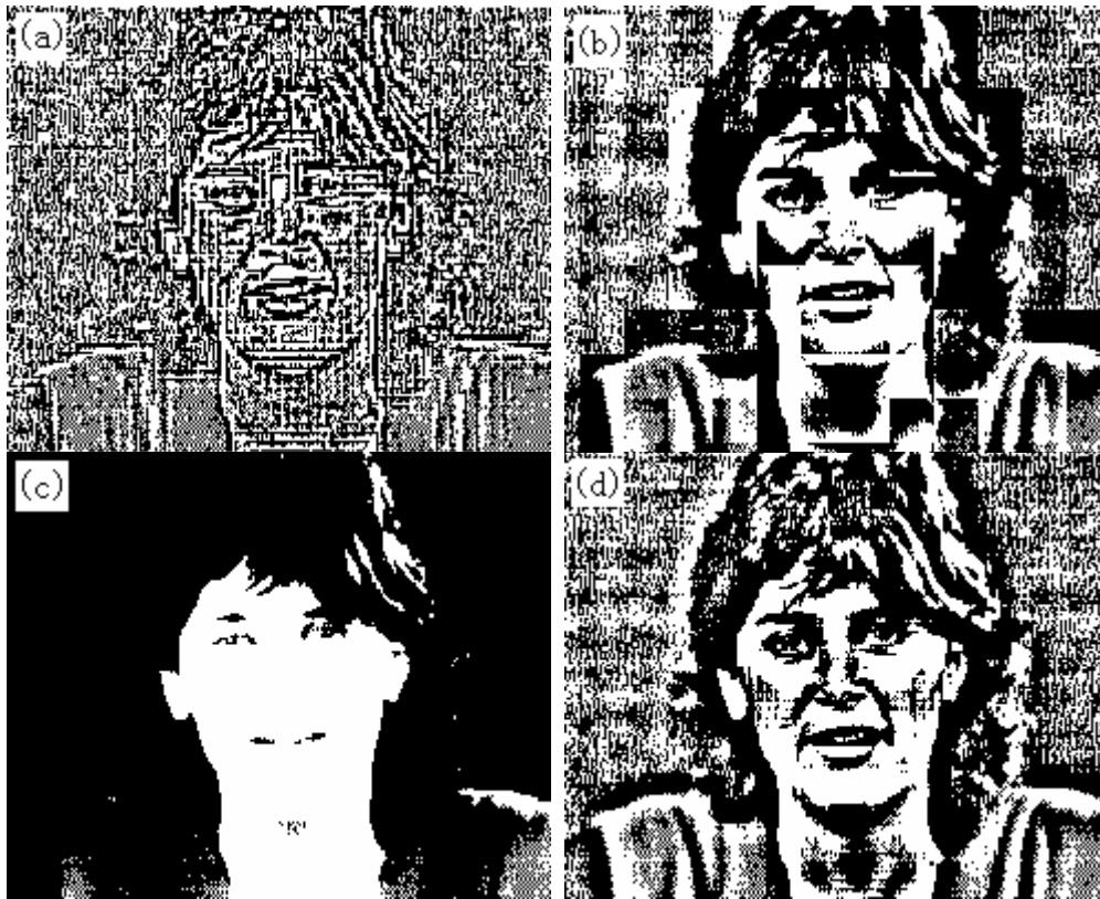
Fig. 4. 1BT transformed bit-planes using (a) BMT with block size 4 \times 4 ; (b) BMT with block size 20 \times 20 ; (c) BMT with block size 352 \times 288 ; (d) OWT with block size 4 \times 4 and window size 22 \times 22 .
