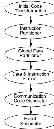
Figure 2: Phase ordering of the basic block orchestrator.
