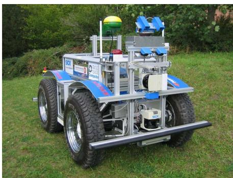
**Figure 1.** RAVON, the Robust Autonomous Vehicle for Off-road Navigation.
