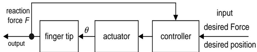
Fig. 7. Block diagram of force and position control of fingers.
