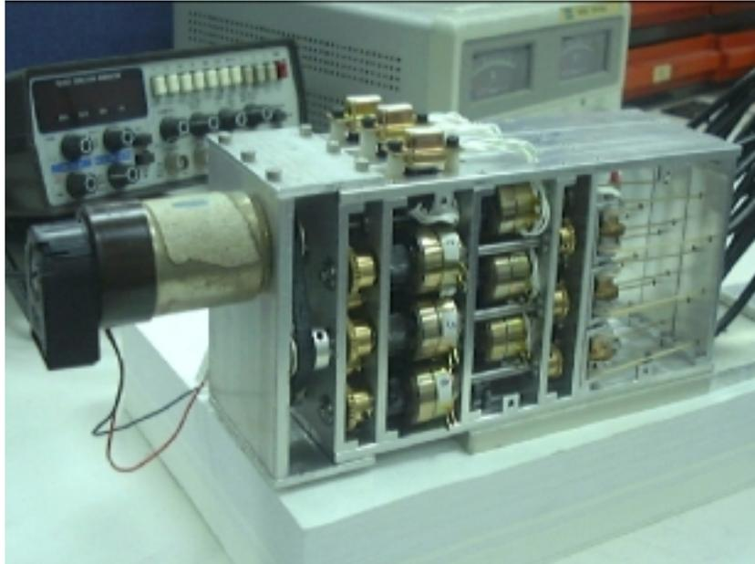
Fig.3. Single motor driven actuator.
