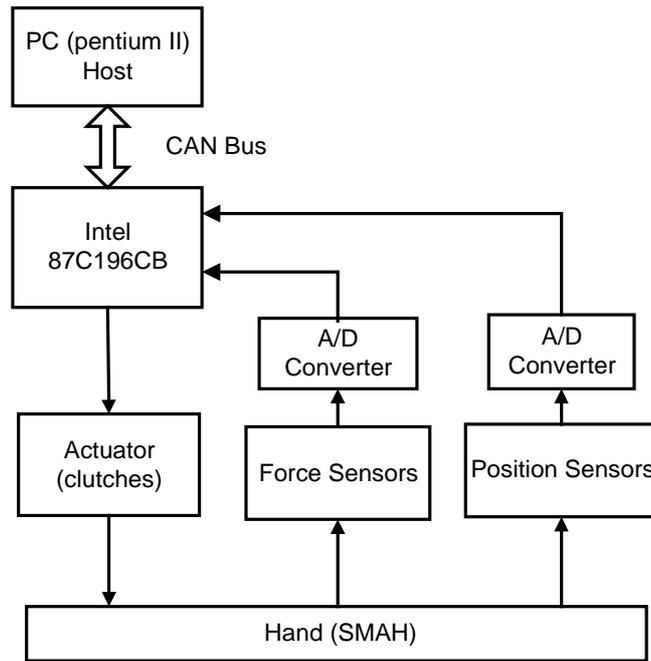
Fig. 5. The hardware Architecture of the Hand
