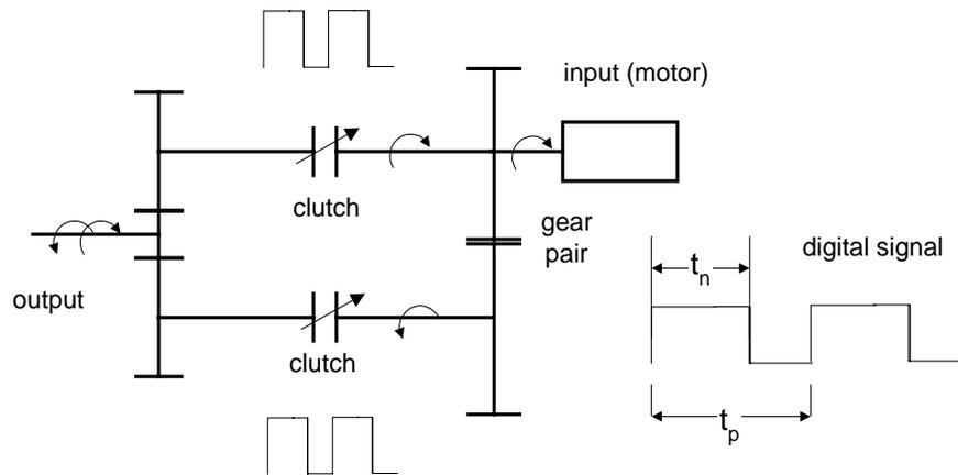
Fig. 6. Schematic chart of motion transmission through clutches.
