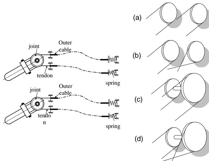
Fig. 2. DOF change in two joints, (1) two DOFs using cases (a) or (b), (2) one DOF using cases (c) or (d).
