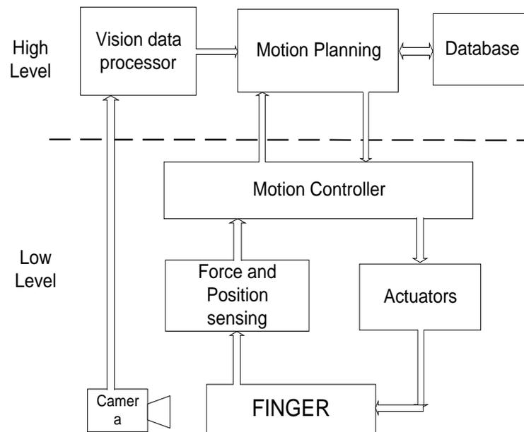
Fig. 4. Control architecture of the hand SMAH
