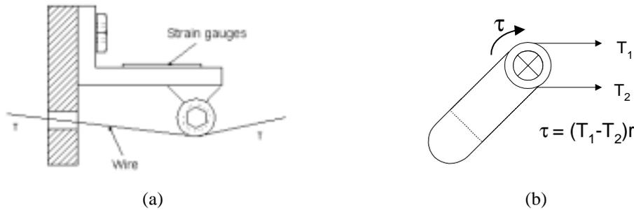
Fig. 8. Measuring method of joint torque, (a) measure wire tension, (b) calculate torque.
