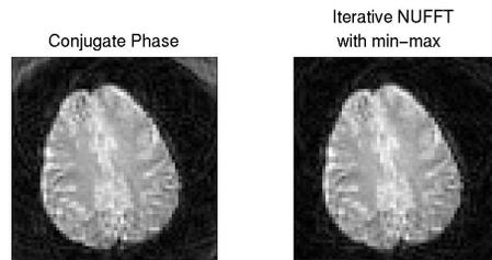
**Fig. 6.** Conjugate phase and iterative image reconstructions. The time for the full conjugate phase was 6.96 s and the time for five iterations of the iterative reconstruction was 5.45 s using  $L = 10$ .
