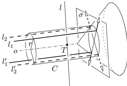
Figure 6: The two lines from Figure 5 can be generated by selecting four pixels from an image of the scene reflected by a conical mirror
