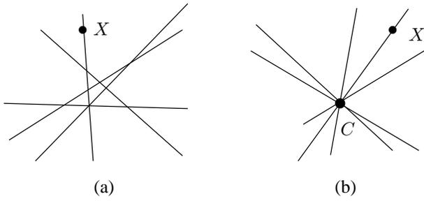
Figure 1: (a) A camera is a set of rays in  $P_3$ . (b) A central camera is a set of all rays incident with one point – the projection center  $C$
