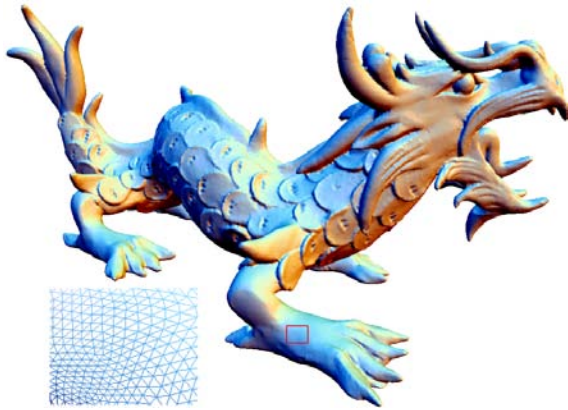
Figure 11: Reconstruction of the XYZ Dragon model (3.6M points - 53.298 sec). Close-up on the semi-regular mesh produced by our algorithm.
