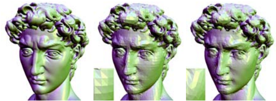
Figure 4: Hierarchical mesh simplification with L^2 error bounded at 2.10^{-3} . Left: Original object (7M triangles). Middle: Octree simplification (1.75 sec. - 62856 triangles). Right: VS-Tree simplification (1.20 sec. - 52024 triangles).
