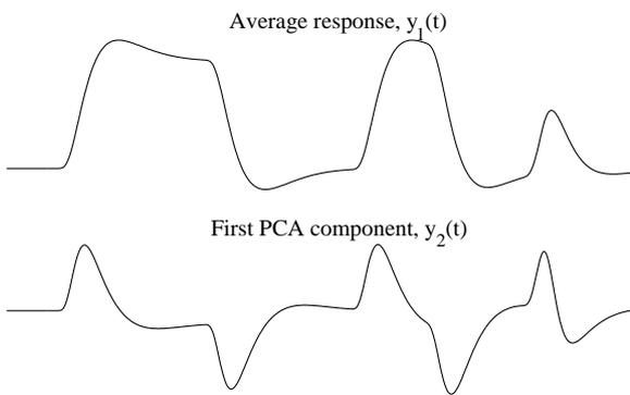
Figure 4: The resulting temporal basis functions when PCA has been applied to simulated responses similar to the examples in Fig. 3
