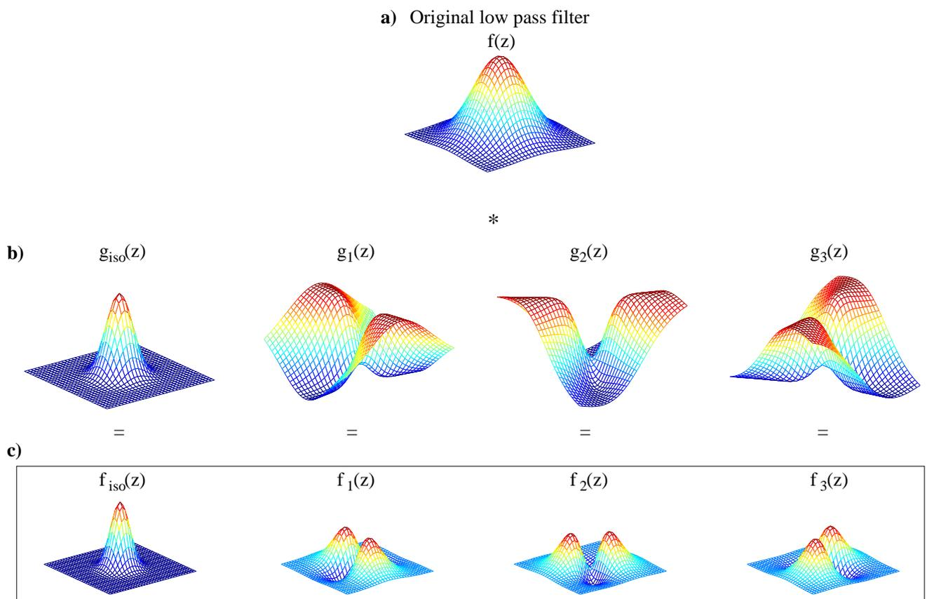
Figure 1: The construction of a set of 2D spatial basis filters. In a), a smoothing filter traditionally used for filtering the fMRI images is shown. In b), four weight functions divide the filter space into four parts. These functions sum to one in every point. In c) the final spatial basis functions are obtained by weighting the original filter with the weight functions.
