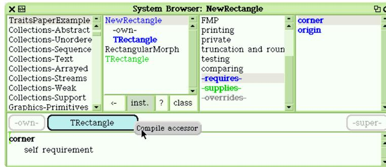
Fig. 4. Compiling an accessor for an instance variable in the new Rectangle class.
