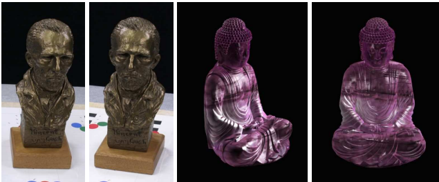
Figure 1: Scenes with strong specularities or made of translucent materials with no distinct point features are a challenge to most stereo algorithms.
