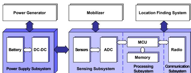
FIG. 2: Architecture of a typical wireless sensor node.
