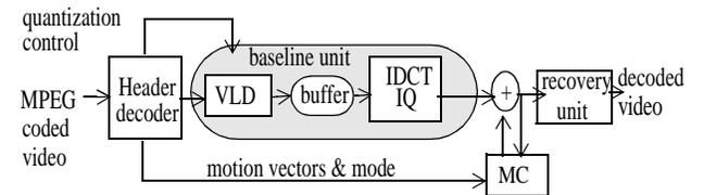
Fig.3 The block diagram of the MPEG-2 decoder
