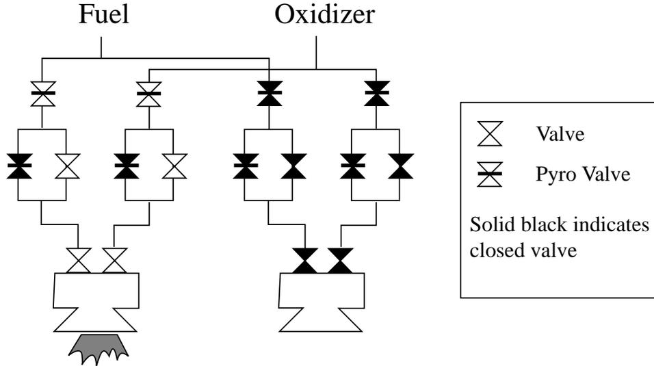
Figure 10: Simplified schematic of Cassini spacecraft propulsion system.
