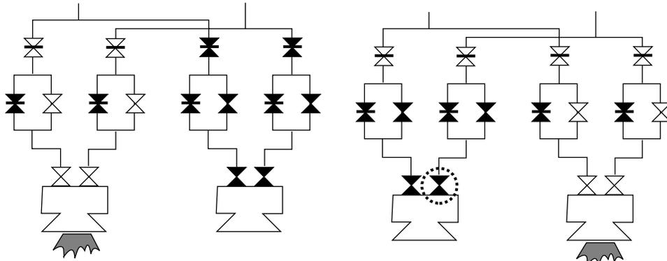
Figure 12: Different configurations that achieve thrust. The circled valve has failed.
