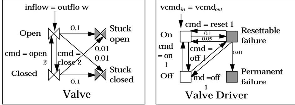
Figure 13: Transition systems for a valve and a valve driver. Shaded modes are failure modes. Fractional numbers represent transition probabilities and whole numbers represent transition costs.
