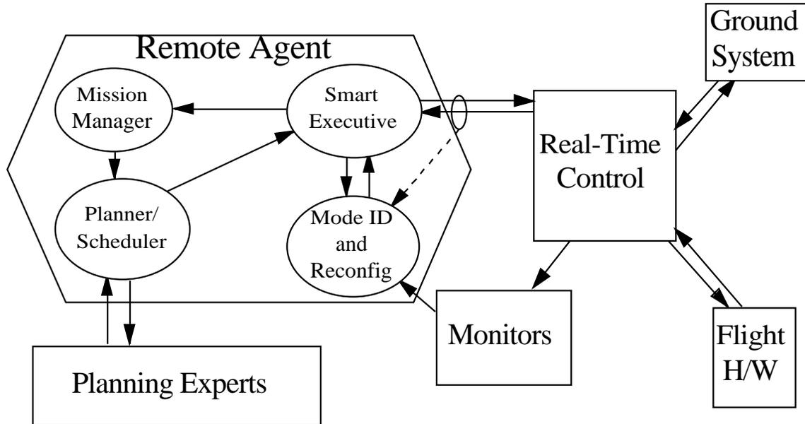
Figure 2: Remote Agent architecture embedded within flight software.
