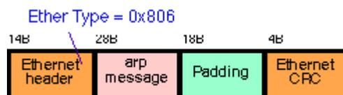
Figure 4: ARP message in an Ethernet header
