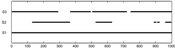
Fig. 4. **Contact Data** Ground contact information is plotted for struts  $S_1$ ,  $S_2$  and  $S_3$  for 1000ms. Dark portions of the lines indicate when a strut is in contact with the ground, and the absence indicates loss of ground contact.
