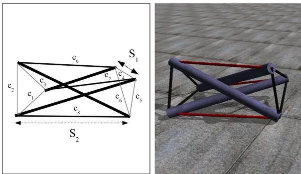
Fig. 1. a) Schematic of the 3-prism tensegrity structure. The thick black lines indicate the struts. The thin grey lines indicate the cables at the two ends of the prism. These are of length  $S_1$ . The thin black lines indicate the transverse cables connecting the two sides of the prism. These are of length  $S_2$ . b) The robot TR-3, based on the 3-prism tensegrity structure, in simulation.
