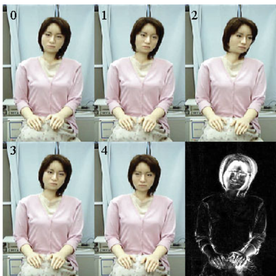
Figure 9: Micro movements of the android. Five snapshots and the movements (bottom right)
