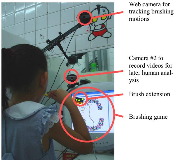
**Figure 4. The brushing tracker uses a web camera anchored on a mirror to track an LED-coded toothbrush extension. The brushing game appears on an LCD display**
