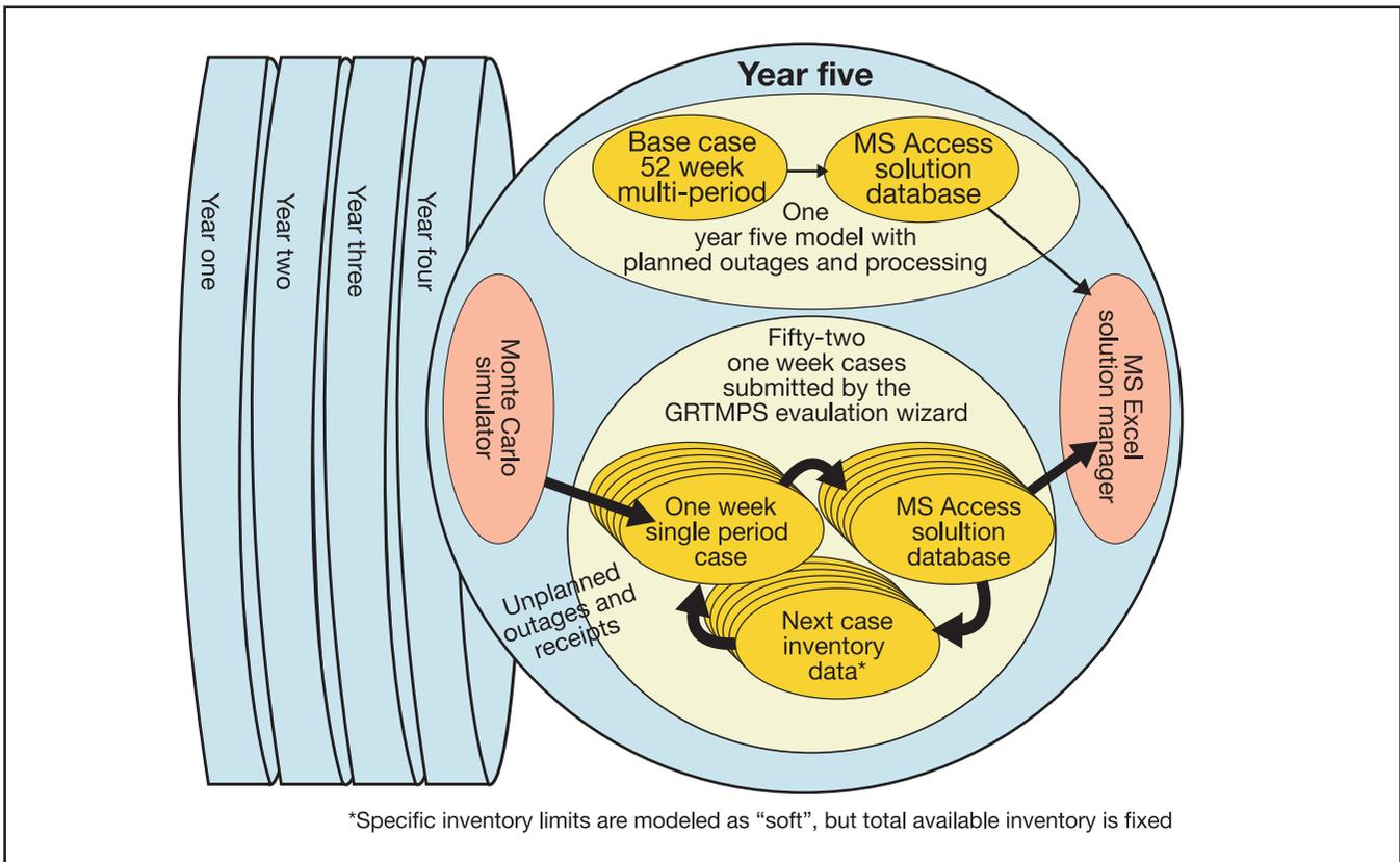
Figure 2 Tank farm simulation model structure
