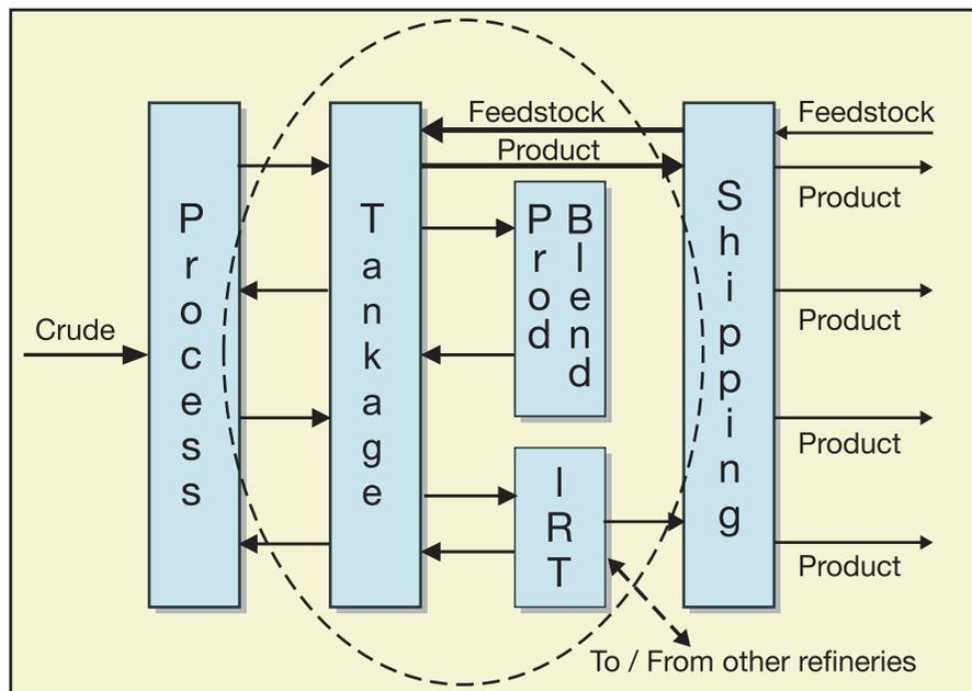
Figure 1 Typical refinery block flow diagram
