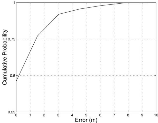
Figure 4. Bulk cumulative error distribution for 1307 packets over 22 poses in hallway 1 in our test area (see figure 1, the building map) localized using the position of maximum probability as calculated by direct application of Bayes' rule.
