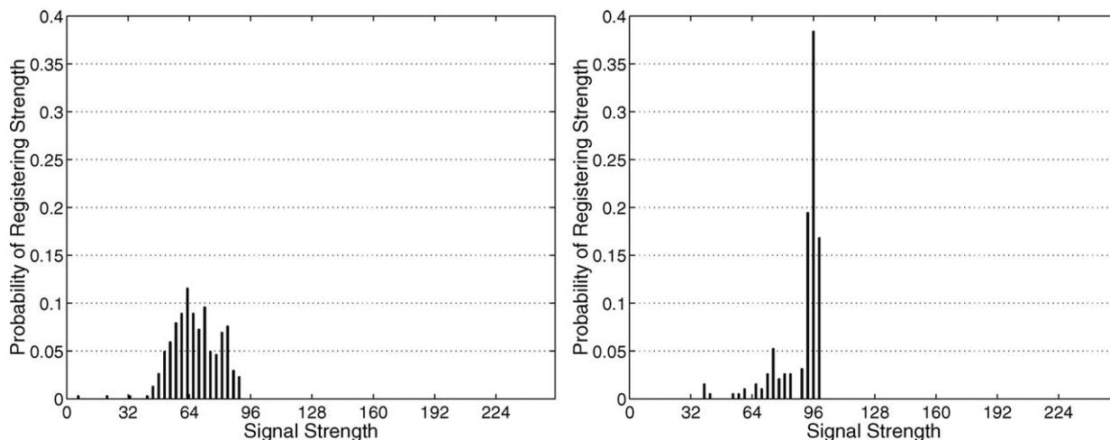
Figure 2. Samples of signal strength taken at the same positions facing opposite directions. The signal strength values indicated are the raw values returned by the network interface.
