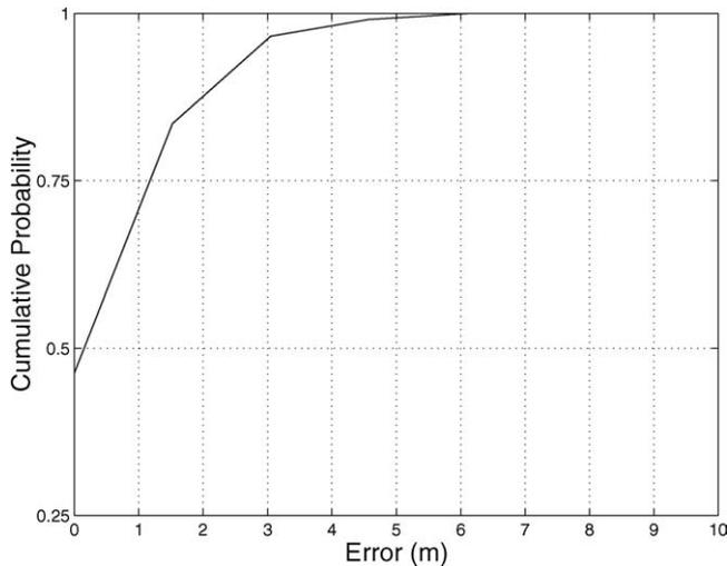
Figure 5. Bulk cumulative error distribution for 1465 packets over 22 poses in hallway 1 in our test area (see figure 1, the building map) localized using the position of maximum probability as calculated by merging distributions over a one second window.
