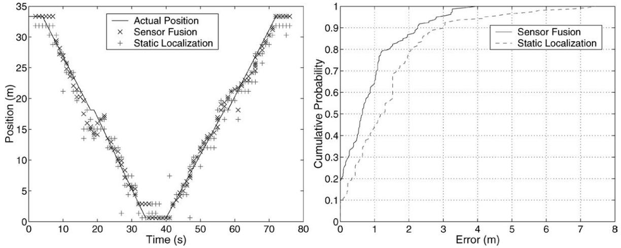
Figure 6. Tracking a round-trip walk of hallway 1 in our test area (see figure 1, the building map). Measured error for the track, shown on the right graph, is at most one meter with probability 0.64, an improvement of 45% over static localization. This improvement is illustrated in the actual tracking performance, shown in the left graph.
