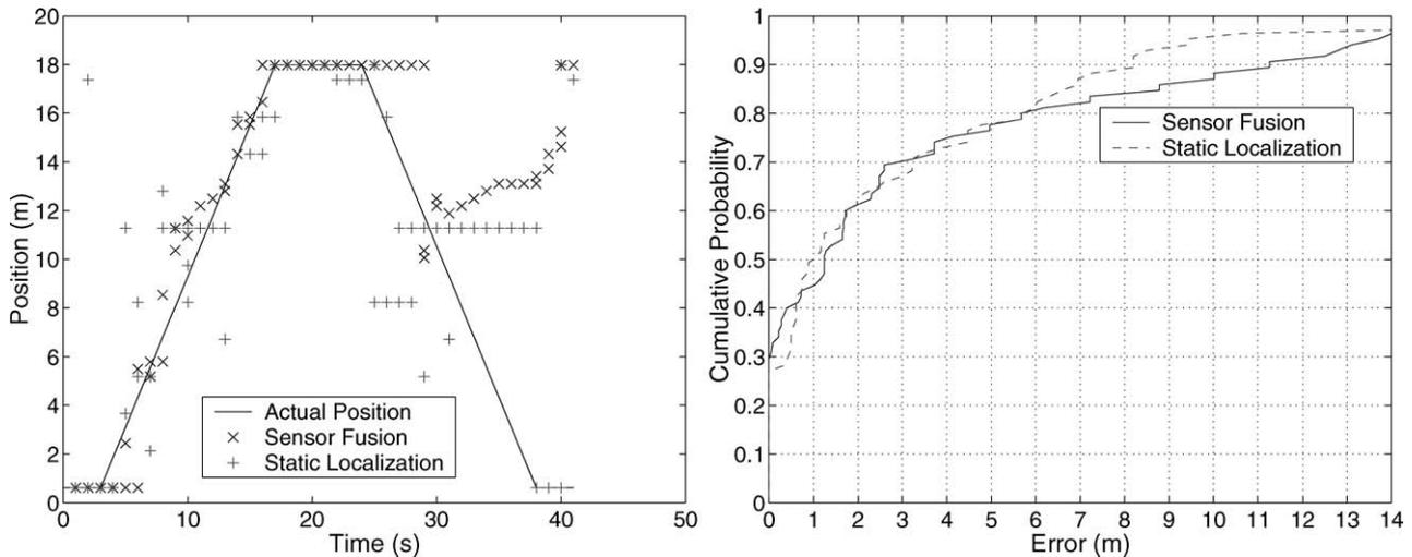
Figure 9. Tracking a round-trip walk of hallway 3 in our test area (see figure 1, the building map). Sensor fusion did not provide a significant improvement in error, and at times increased error, as shown in the right graph. However, as shown in the left graph, the raw data was already extremely noisy in this case.
