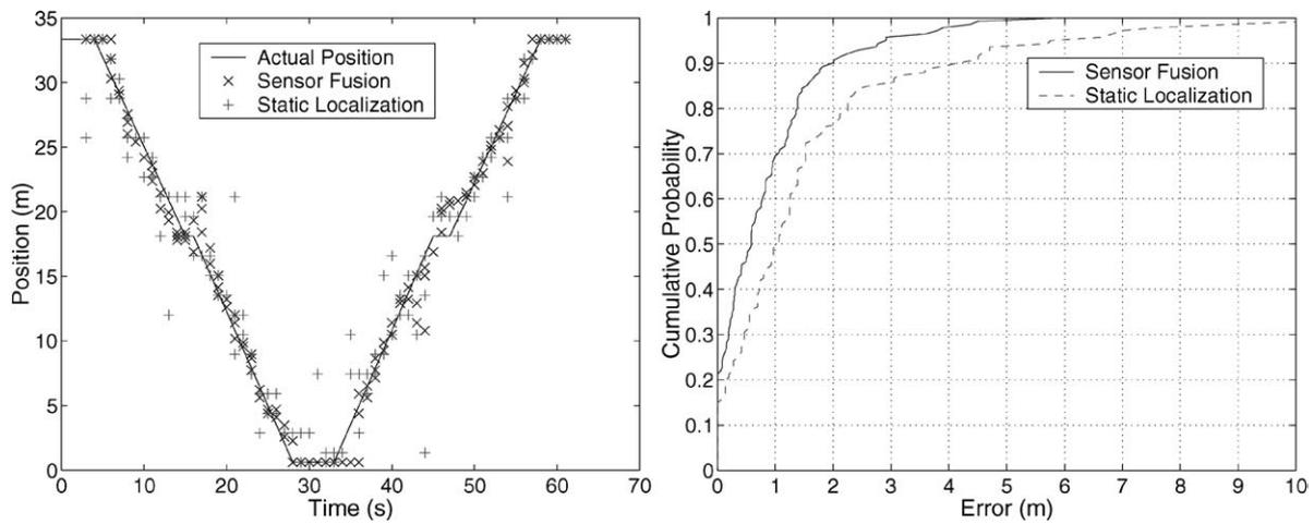
Figure 7. Tracking a round-trip walk of hallway 2 in our test area (see figure 1, the building map). Measured error for the track, shown on the right graph, is at most one meter with probability 0.7, an improvement of 40% over static localization. This improvement is illustrated in the actual tracking performance, shown in the left graph.
