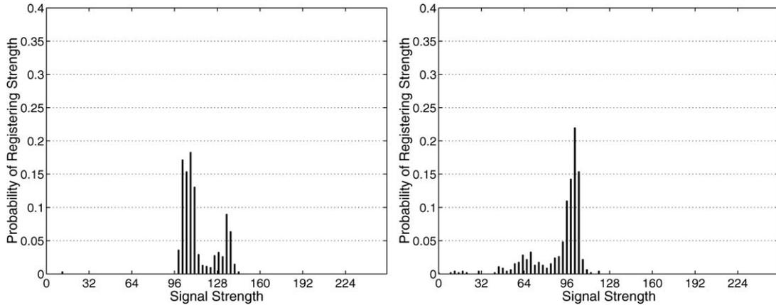
Figure 3. Samples of signal strength distributions of two different base stations, measured simultaneously from one location. The signal strength values indicated are the raw values returned by the network interface.
