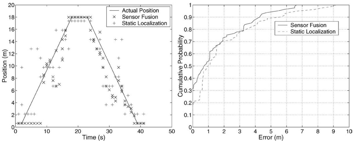
Figure 8. Tracking a round-trip walk of hallway 4 in our test area (see figure 1, the building map). While sensor fusion provided some improvement, it was not significant. As shown in the left graph, when static localization was significantly off, so was sensor fusion, but when static localization appears to track actual movement, sensor fusion is surprisingly accurate despite the noise.
