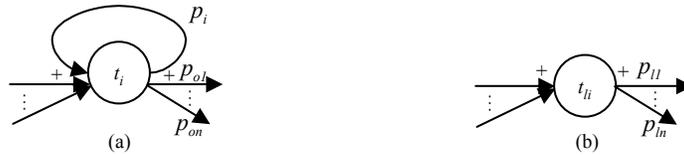
**Figure 6 – Simple loop system reduction**
