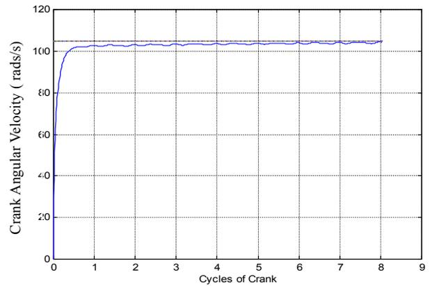
**FIGURE 9(b):** Crank Angular Velocity Vs. Cycles of Crank (Time represented in units of cycles of crank) [Motion Profile (iii)]
