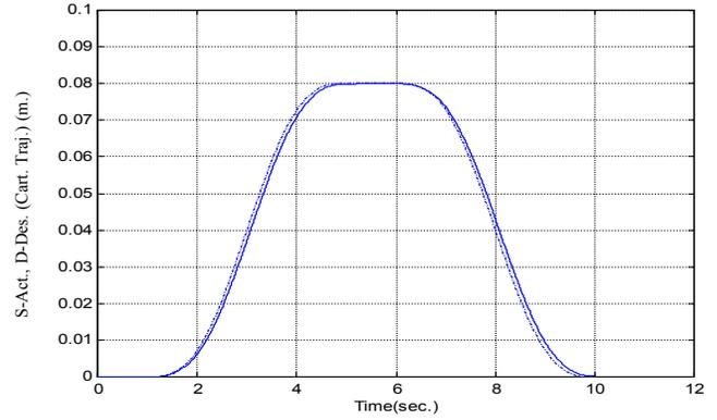
**FIGURE 3:** Desired and Actual Position of the Slider (Cartesian) for the first Crank Cycle [Motion profile (i) in Table 1]
