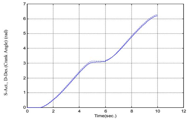
**FIGURE 5:** Desired and Actual Angular Position of Crank from 0 rad – 2pi rad. ( 1<sup>st</sup> Cycle) [ Motion profile (i) in Table 1]
