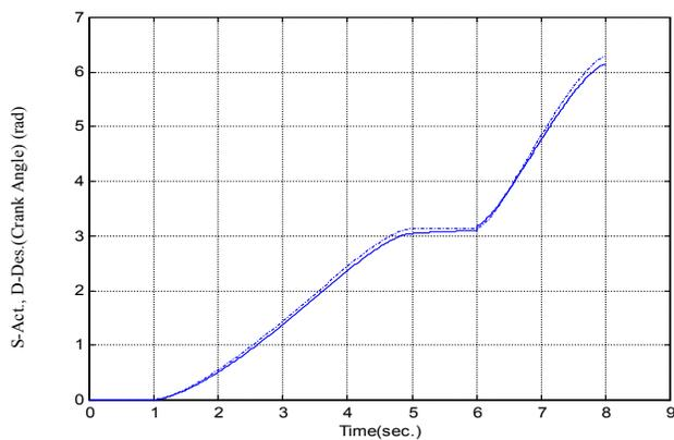
**FIGURE 8:** Desired and Actual Angular Position of Crank from 0 rad –  $2\pi$  rad. (1<sup>st</sup> Cycle) [Motion profile (ii) in Table 1]
