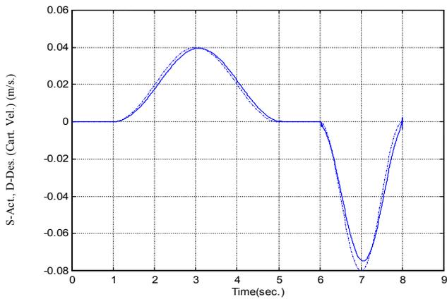
**FIGURE 7:** Desired and Actual Velocity of the Slider for the first Crank Cycle [Motion profile (ii) in Table 1]
