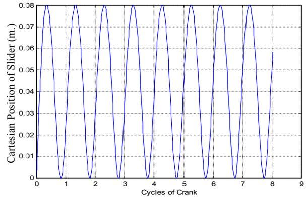
**FIGURE 9(a):** Slider Motion Vs. Cycles of Crank (Time represented in units of cycles of crank) [Motion Profile (iii)]
