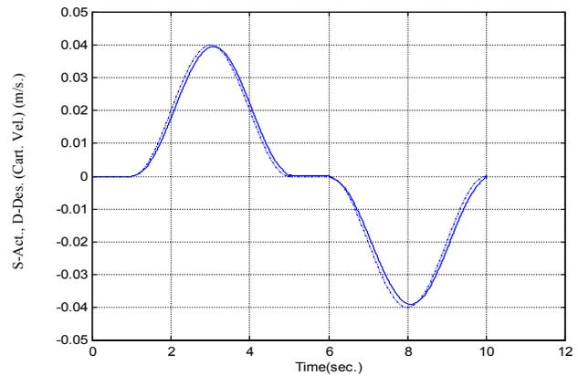
**FIGURE 4:** Desired and Actual Velocity of the Slider for the first Crank Cycle [ Motion profile (i) in Table 1]
