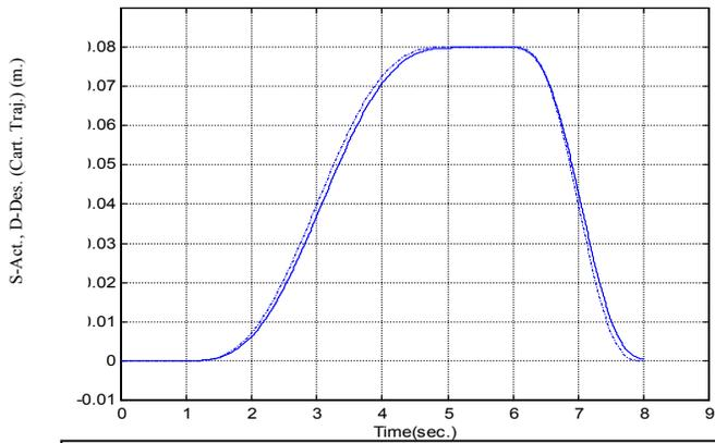
**FIGURE 6:** Desired and Actual Position of the Slider (Cartesian) for the first Crank Cycle [Motion profile (ii) in Table 1]
