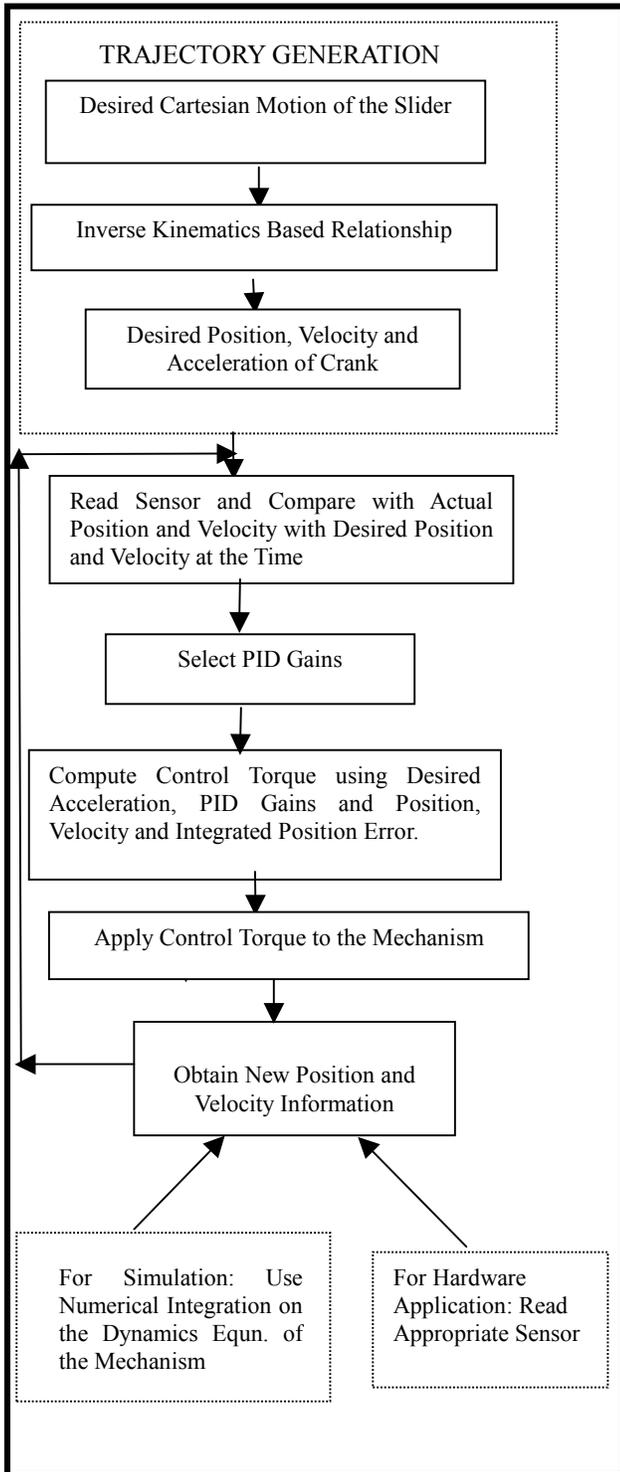
**Figure 2 :** Simulation and Control Scheme
