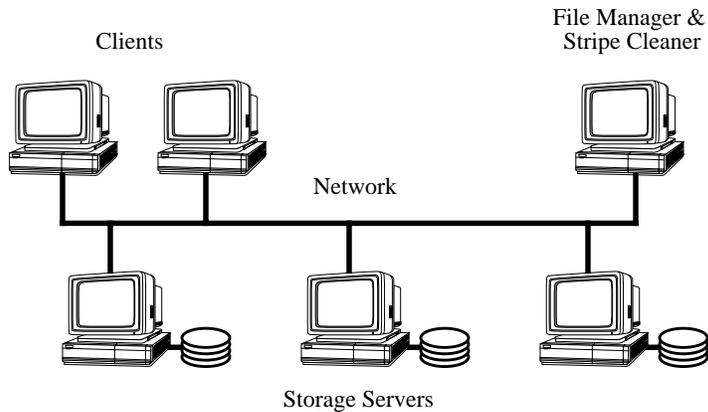
**Figure 5: Zebra schematic.** Clients run applications; storage servers store data. The file manager and the stripe cleaner can run on any machine in the system, although it is likely that one machine will run both of them.
