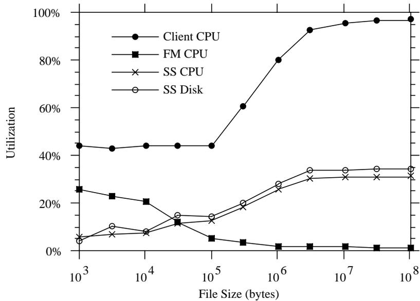
**Figure 8. Read resource utilizations.** The curves are similar in shape to those for writing, except that the knees occur at larger file sizes. The storage server utilizations were measured on one of the five servers in the system. For small files the loads were not equal on all of the servers, causing the fluctuations in the curves. The standard deviations for all measurements are less than 2%.
