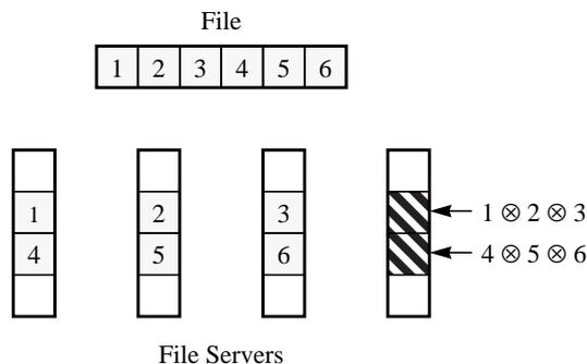
**Figure 2. File-based striping for a large file.** The file is divided up into stripe fragments that are distributed among the servers. One fragment of each stripe contains the parity of the stripe's contents.
