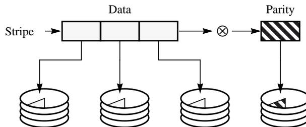
**Figure 1. Striping with parity.** The storage space of a RAID disk array is divided into stripes, where each stripe contains a striping unit on each disk of the array. All but one of the striping units hold data; the other striping unit holds parity information that can be used to recover after a disk failure.
