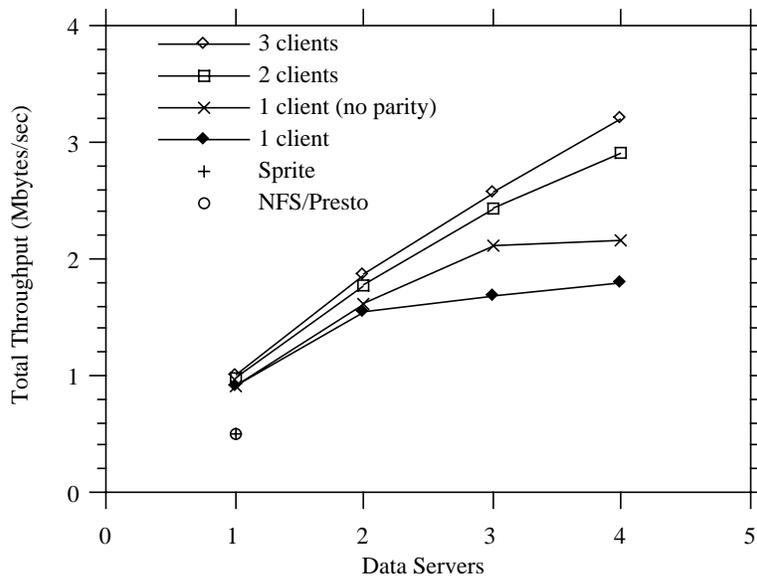
**Figure 9. Total system throughput for large file writes.** Each client ran a single application that wrote a 12-Mbyte file and then flushed the file to disk. In multi-server configurations data were striped across all the servers with a fragment size of 512 Kbytes. Each Zebra configuration also included a parity server in addition to the data servers. The maximum standard deviations are 0.06 Mbytes/second for Zebra, 0.01 Mbytes/second for Sprite, and 0.16 Mbytes/second for NFS.
