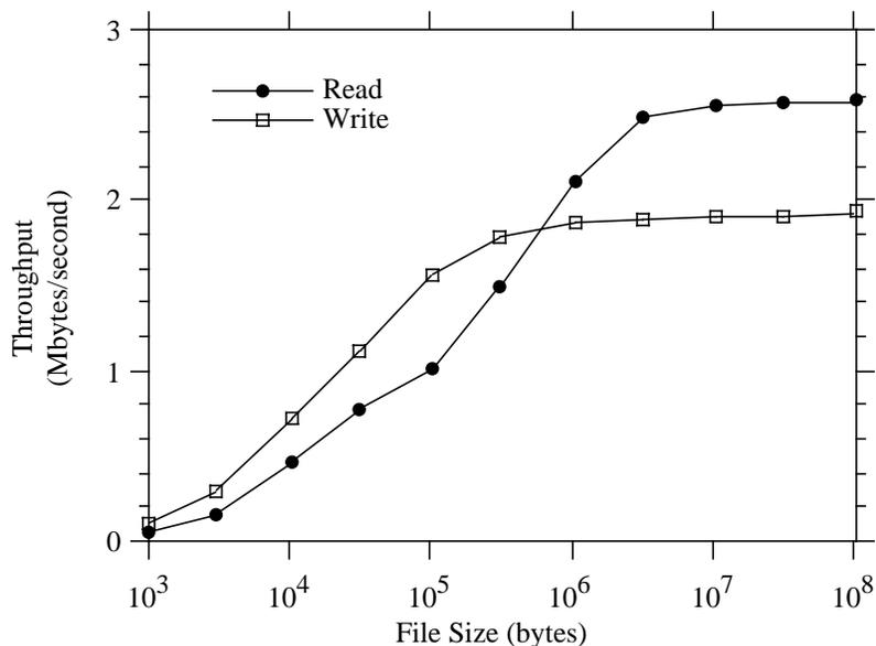
**Figure 6. Throughput vs. File Size.** A single client reads or writes files of varying size to five storage servers. Writing small files is faster than reading due to Zebra's ability to batch small writes; writing of large files is slower than reading due to the parity computation.
