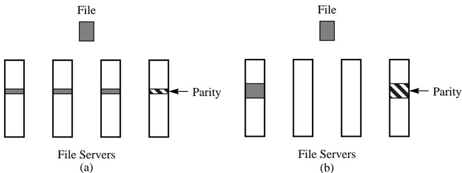
**Figure 3. File-based striping for a small file.** In (a) the file is striped evenly across the servers, resulting in small fragments on each server. In (b) the entire file is placed on one server but the parity requires as much space as the file data.
