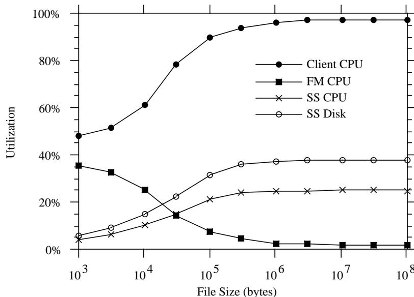
**Figure 7. Write resource utilizations.** For small files the time required to open and close the files causes low client utilization and high file manager utilization (this effect is described in more detail in Section 8.4); for large files the client CPU saturates. The storage server utilizations were measured on one of the five servers in the system. The maximum standard deviation for the measurements is 3%.
