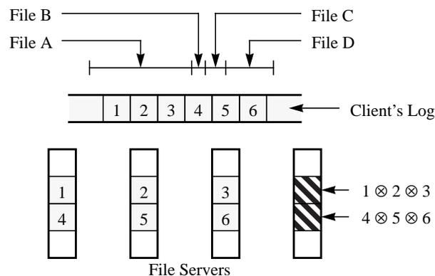
**Figure 4. Log-based striping in Zebra.** Each client forms its new file data into a single append-only log and stripes this log across the servers. In this example file A spans several servers while file B is stored entirely on a single server. Parity is computed for the log, not for individual files.
