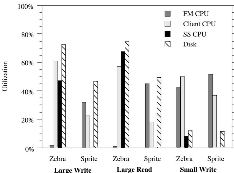
**Figure 12: Resource utilizations.** Utilizations of the file manager (FM) CPU and disk, client CPU, storage server (SS) CPU, and the disk during the previous three benchmarks. The Zebra system consisted of a single client, a single file manager, and two storage servers, one of which stored parity; the Sprite system consisted of a single client and a single file server, which served as both file manager and storage server. The standard deviations for all measurements are less than 1%.
