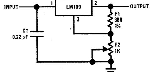
Fig. 10. Using the LM109 as an adjustable-output regulator.
