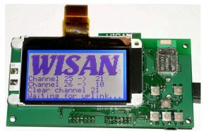
Fig. 3. Front and rear view of a WISAN coordinator.
