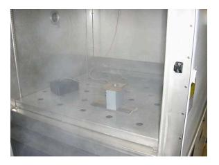
Fig. 5. WISAN sensor box in environmental chamber.
