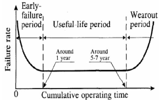
Figure 2: Lifecycle failure pattern for hard drives [33].
