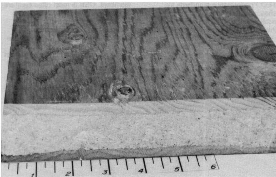
Figure 4—Specimen of a composite plywood panel. The edge has been bevel-cut to accentuate the wood-particle core. (Numbered scale in inches.) (M 150 063)
