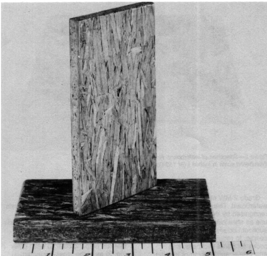
Figure 3—Two small specimens of oriented strandboard. This shows the board's three-layer construction and alignment of strands in each layer. (Numbered scale in inches.) (M 150 062)
