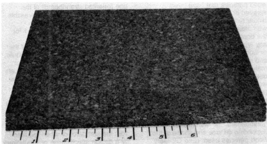
Figure 1—Specimen of underlayment particleboard. (Numbered scale in inches.) (M 150 064)
