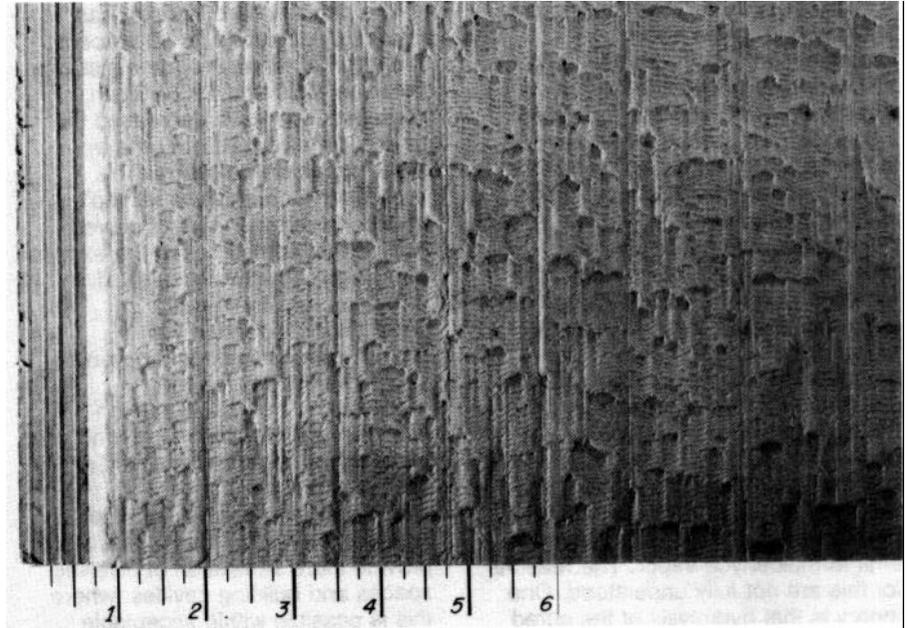
Figure 5—Specimen of grade 2-M-1 board produced for vertical exterior siding. This specimen has a textured surface and is overlaid with phenolic-resin impregnated paper. (Numbered scale in inches.) (M 150 061)
