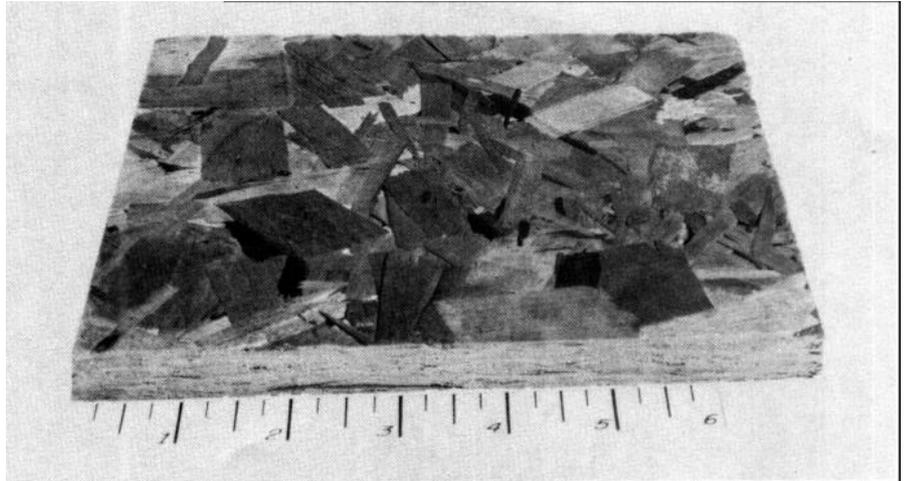
Figure 2—specimen of waferboard. Note the wide wafers, (Numbered scale in inches.) (M 150 065)
