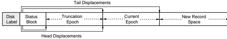
This figure shows the organization of a log during epoch truncation. The current tail of the log is to the right of the area marked "current epoch". The log wraps around logically, and internal synchronization in RVM allows forward processing in the current epoch while truncation is in progress. When truncation is complete, the area marked "truncation epoch" will be freed for new log records.
