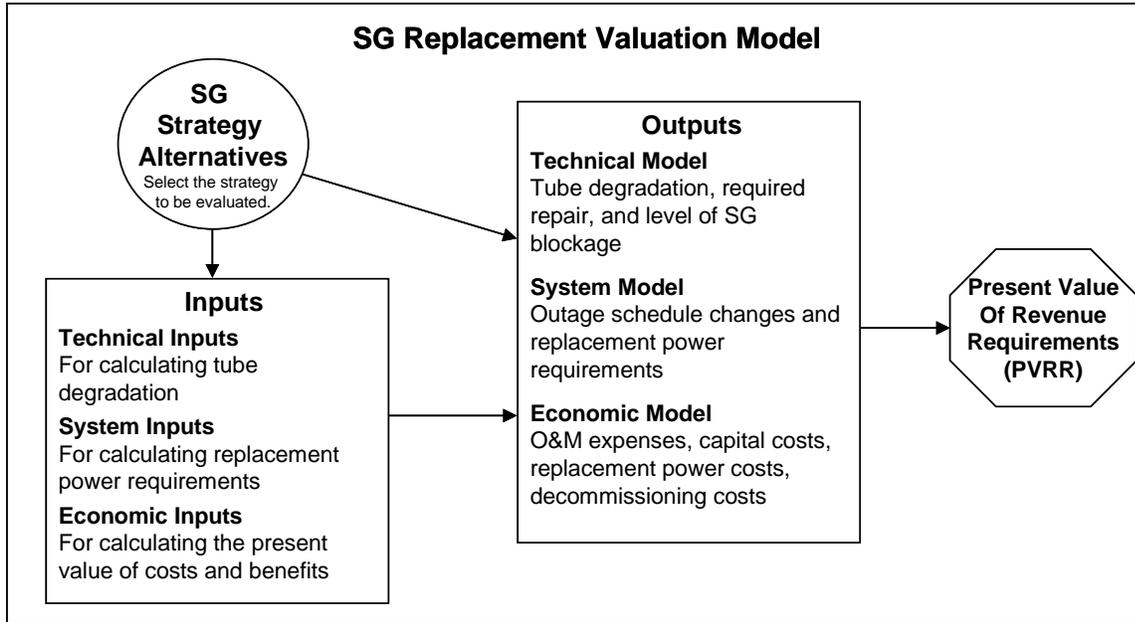
Figure 1: Pacific Gas and Electric Company overall steam generator model structure
