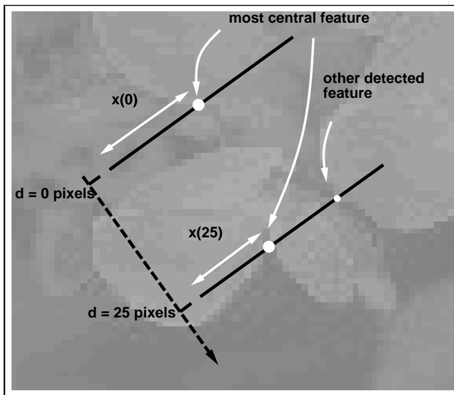
Figure 6: **Investigating feature correlation.** The top solid black line is a measurement line positioned randomly on a typical background image. The value of the random process  $x(d)$  is the offset of the most central detected feature after the initial measurement line has been displaced by  $d$  pixels in the direction of its normal.
