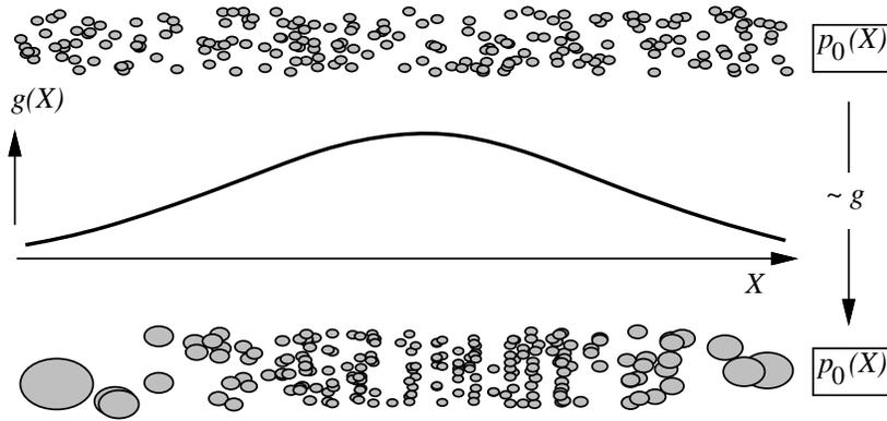
Figure 11: **Weighted resampling.** A uniform prior  $p_0(X)$ , represented as a particle set (top), is resampled via an importance resampling function  $g$  to give a new, re-weighted particle set representation of  $p_0$ . Note that these are one-dimensional distributions; the particles are spread in the  $y$ -direction only so they can be seen more easily.
