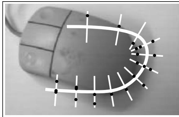
Figure 2: **Measurement methodology.** The thick white line is  $\mathbf{x}$  — a mouse-shaped contour in some hypothesised configuration. The thin lines are *measurement lines*, along which a one-dimensional feature detector is applied. Black dots show the output of the feature detector, which in this case responds to rapid changes in intensity — one-dimensional edges. Note that many spurious edges are generated by shadows, or more generally by clutter in the image.
