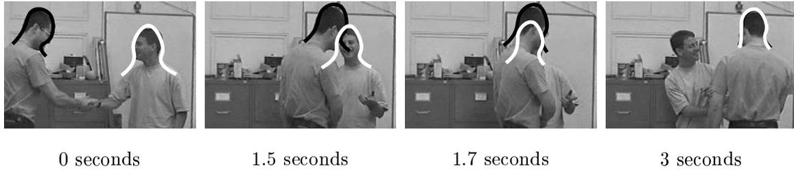
Figure 1: **With an observation model designed for one target, two trackers initialised in distinct configurations eventually lock on to the one target which best fits the model.** The objective is to derive an observation model which does not permit the presence of two targets to be inferred from measurements of only one.
