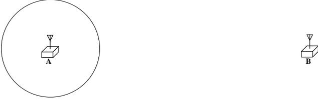
Figure 5: Region of *respect neighbor* constraint on packet scheduling. A station would have to be inside the circle for a transmission from A to B to significantly raise the level of noise at its receiver. In those rare cases, Station A must respect (by not overlapping) the receive windows of any stations inside the circle when scheduling transmissions to Station B.
