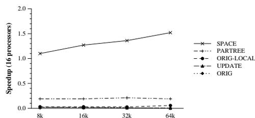
Figure 14: Speedups for the tree building phase on 16 processors using the page-grained HLRC SVM protocol
