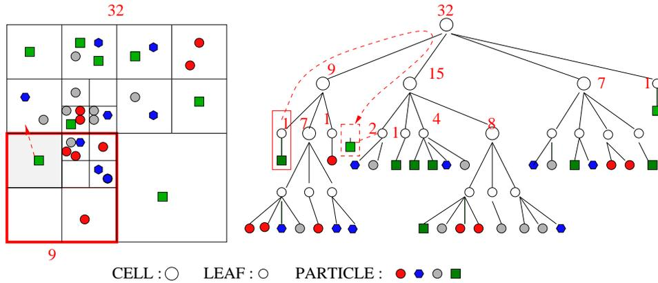
Figure 3: With 4 processors, each subspace at most have 4 particles, the number beside the cells or leaves indicating the number of particles contained in it. The bodies assigned to different processors are represented by different shape.
