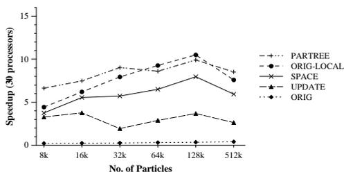
Figure 9: Speedups on Origin 2000 for the tree building phase with 30 processors
