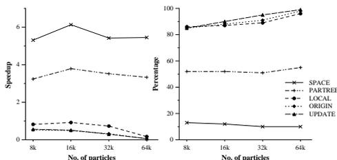
Figure 13: Speedups and Percentage of Time spent in Tree Building on Typhoon-Zero for 16 Processors using the page-based HLRC SVM protocol
