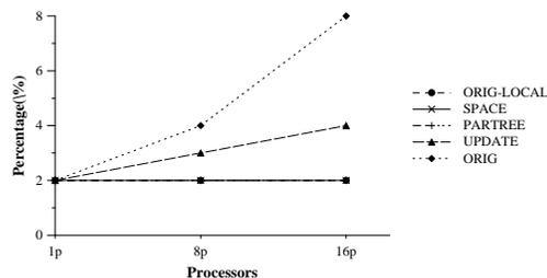
Figure 7: Tree-building cost for 128k particles and 16 processors on SGI Challenge, as a percentage of total execution time. The cost percentages of ORIG-LOCAL, PARTREE and SPACE algorithms are the same
