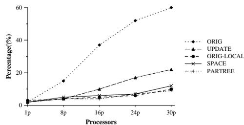
Figure 11: Percentage of execution time spent in Tree Building on Origin 2000 for 512k particles on 30 processors
