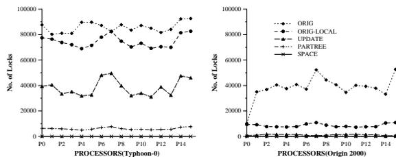
Figure 15: The number of locks of each processor executed in the tree building phase for two time steps with 64k particles using 16 processors
