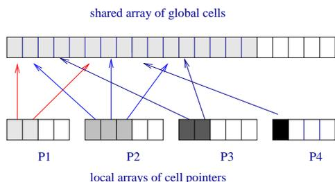
Figure 1: The array of global cells and local arrays of cell pointers used in ORIG Algorithm. The shaded cells are actually used while the blank are not.
