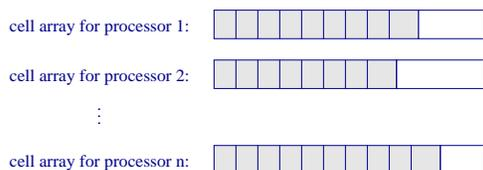
Figure 2: The local cell arrays used in ORIG-LOCAL Algorithm. The shaded cells are actually used while the blank cells are not
