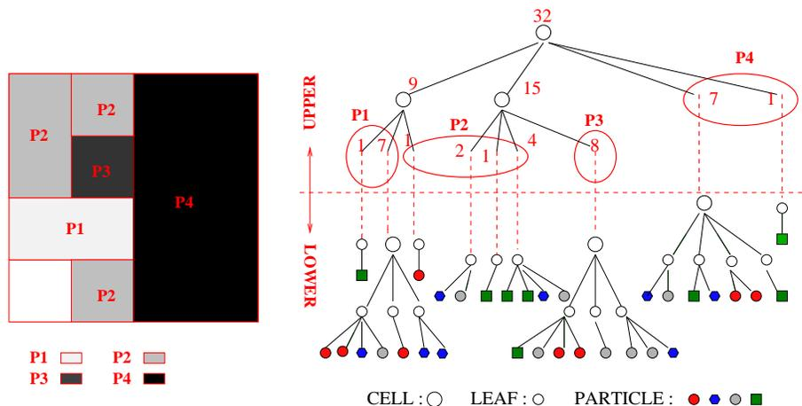
Figure 5: SPACE: the partitioned space and corresponding global tree created using the body distribution in Figure 3
