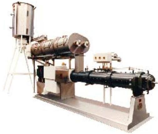
Figure 1 – Twin-screw extrusion cooking system, courtesy of Wenger. The first barrel is a pre-conditioner, used in conjunction with the extruder to increase residence time, reduce mechanical power consumption, and/or increase capacity. A cooling jacket around the extruder, instrumented with thermocouples in various places provides temperature control
