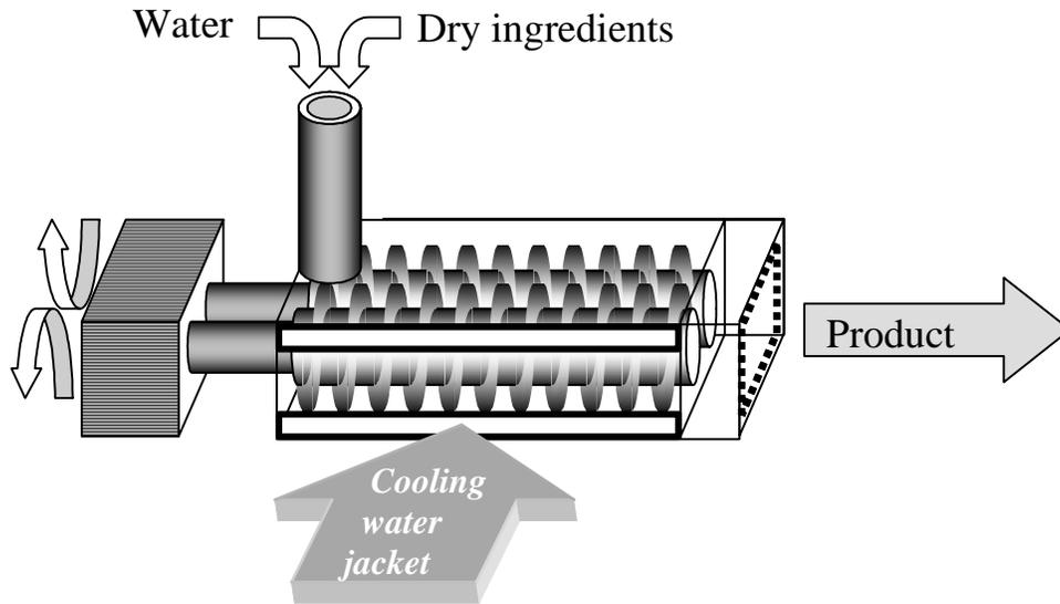
Figure 2 – Simplified schematic of twin-screw extrusion cooker. In food extrusion, the most effective manipulated variables are mass feed rate, moisture content of mass feed, mass and barrel temperatures, and screw speed [51].
