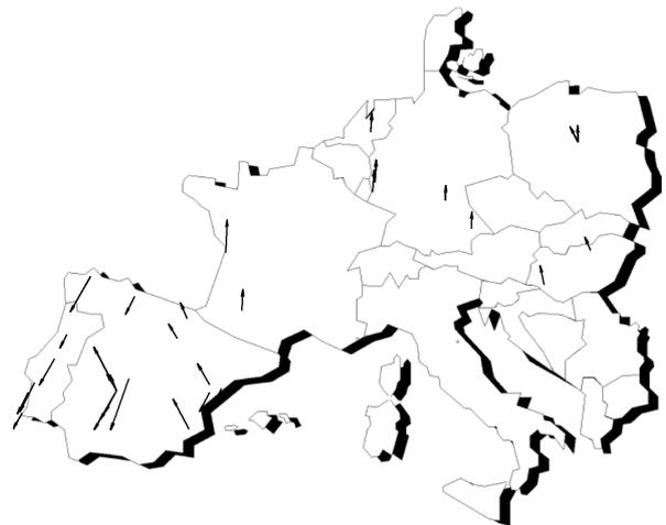
**Fig. 11** Residues of Transfer Function  $\Delta\omega/\Delta V_{\text{excitation}}$  of Global Mode 1
