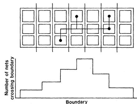
Fig. 2. Construction of a horizontal net-crossing histogram.
