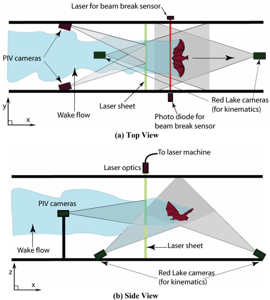
**Figure 2** Schematic of the experimental setup for the measurement in the transverse (Trefftz) plane. The bat flies from left to right and triggers the acquisition sequence by triggering a beam-break sensor. The wake is imaged in a plane behind the animal, after she has passed through.
