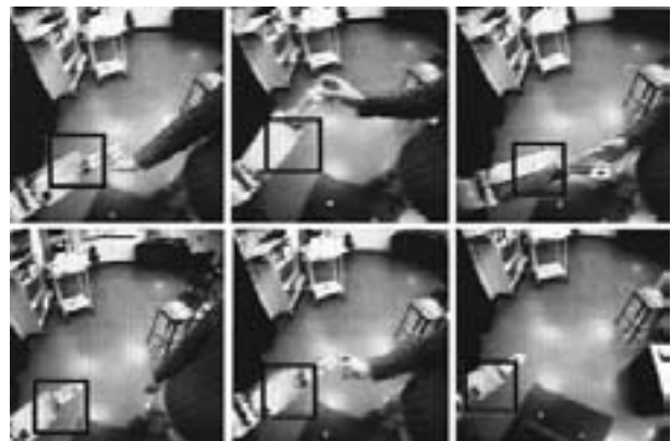
Figure 5 Predicting the location of the arm in the image as the head and arm change position. The rectangle represents the predicted position of the arm using the map learned during a 20-min training run. The predicted position just needs to be sufficiently accurate to initialize a visual search for the exact position of the end effector.
