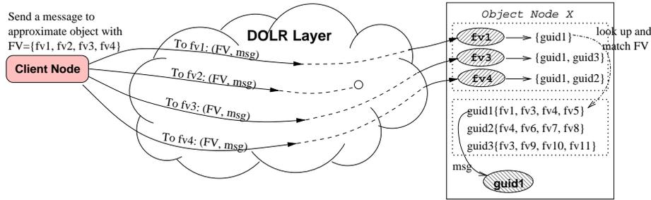
**Fig. 5. Optimized ADOLR location.** Client node wants to route a message to a feature vector  $\{fv1, fv2, fv3, fv4\}$ . It sends message to each identifier  $fv1, fv2, fv3, fv4$ .  $fv2$  doesn't exist, so no object node receives this message. When object node X receives the messages to  $fv1, fv3$  and  $fv4$ , it scans its local storage for all IDs matching  $fv1, fv3$  and  $fv4$ , which is  $guid1$ . Then, object node X sends msg to  $guid1$ .
