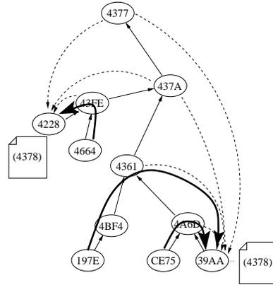
**Fig. 3. Object Location in Tapestry:** Three different location requests. For instance, to locate GUID 4378, query source 197E routes towards the root, checking for a pointer at each step. At node 4361, it encounters a pointer to server 39AA.
