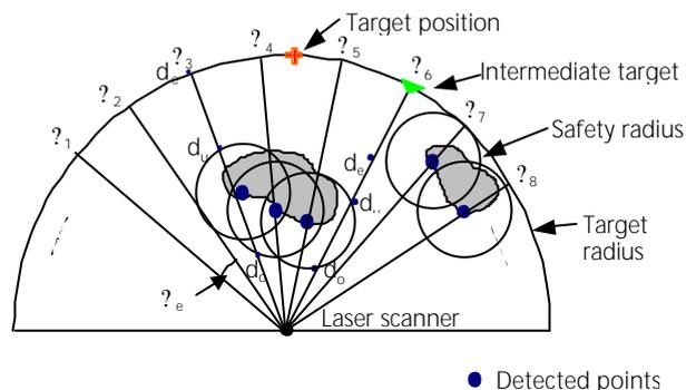
Figure 4. Reactive obstacle avoidance using the "PolarBug" algorithm
