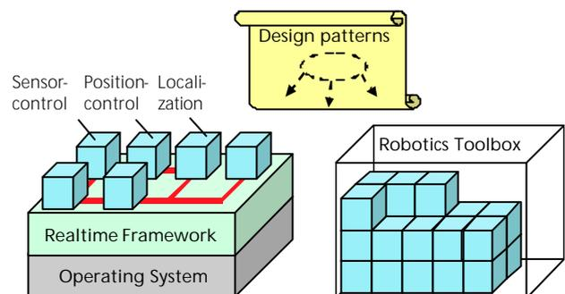
**Figure 2.** Software Architecture
