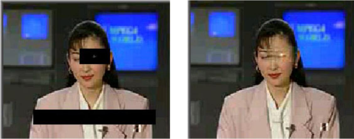
Fig 6. Degraded image (left), error concealed image (right)
