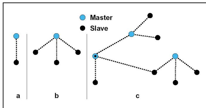
Fig 1 Piconets with a single slave operation (a), a multi-slave operation (b) and a scatternet (c)
