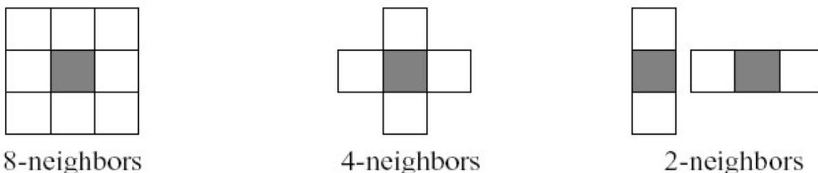
Fig 5.Recovering lost blocks using neighbouring blocks, white blocks are correctly received blocks, dark blocks are lost
