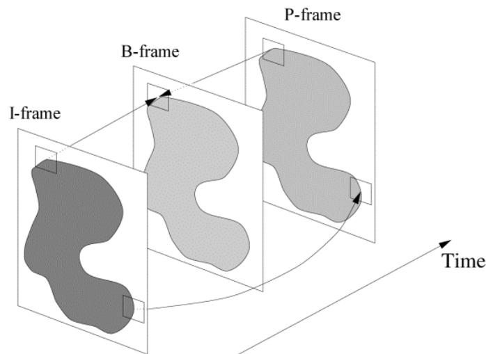
Fig 3.the three modes of frame encoding
